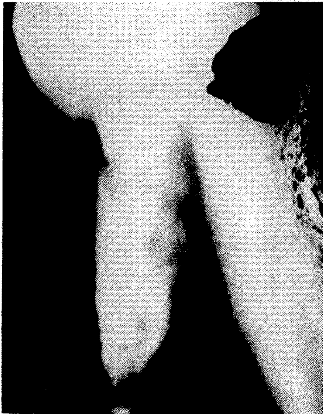
Figure 3. Clay descending through a density stratified brine is slowed at every microstratification surface.
